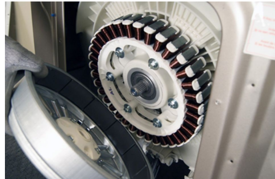
Figure 8: A Direct Drive Radial Flux Motor in a Washing Machine
