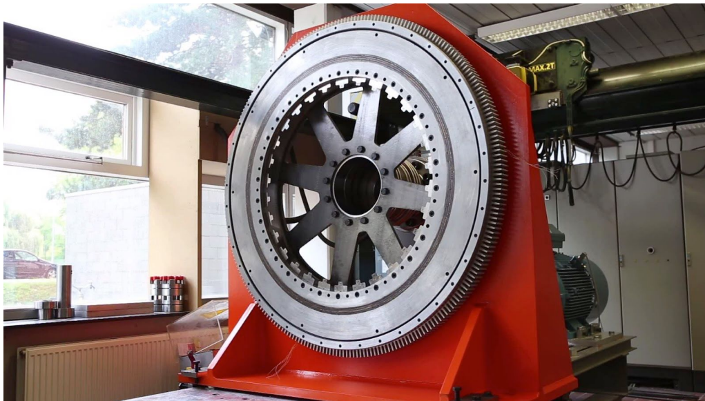
Figure 2: Summer 2017 - Magnax 100-kW 16 kNm Prototype Generator on the test bench check out the youtube video
